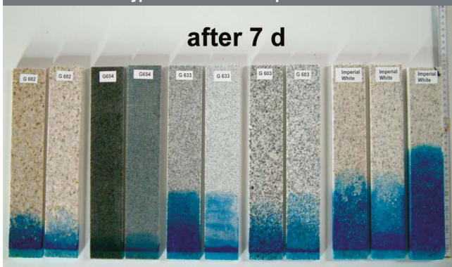
Different stone types show different porosities
